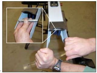
Spread the frame to remove the upper hanger axle. Use equal pressure on both sides.
