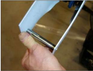
Spread the frame to remove the lower hanger axle.
