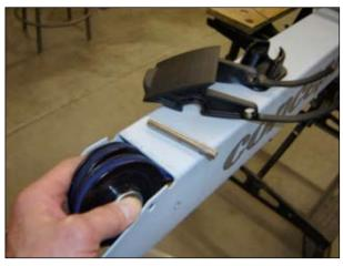
Remove axle from pulleys and mouse. Remove mouse.
