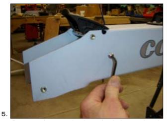
Remove the two shock cord axle button head fasteners.
