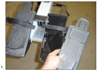
Remove the footplate covers by taking out the 12 philips head screws.
