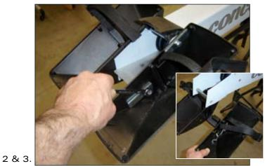
Remove the footplate bellies by taking out the 4 7/16" hex screws and plates.
