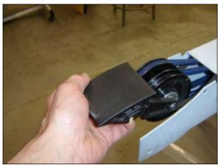
Pull out the mouse, shock cord pulleys and axle.
